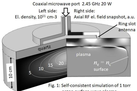
Fig. 1: Self-consistent simulation of 1 torr argon surface-wave plasma
